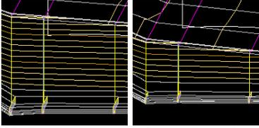
Civil 3-D also revolutionizes the site design and development processes. For example, as the grading centerline is adjusted, Civil 3-D automatically recalculates the height of the retaining wall.
